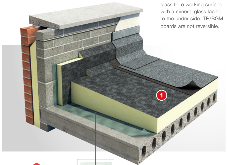
Mineral glass facing to the under side of BGM board.
