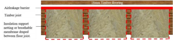
Fully ventilated air space below the timber joist
