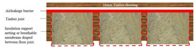
Fully ventilated air space below the timber joist
