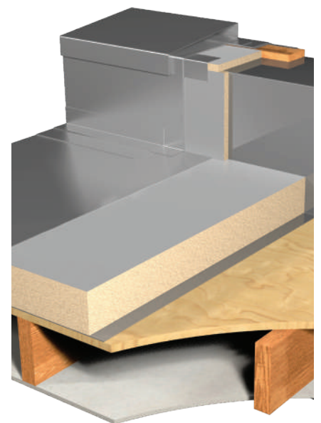
Flat roofs: MFR-DPFR on timber deck
