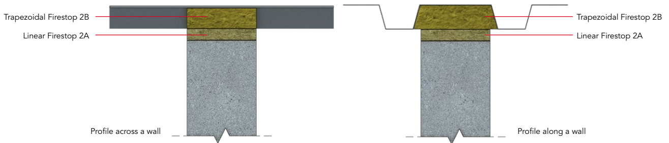
Figure 4 – Profiled metal deck over blockwork wall
