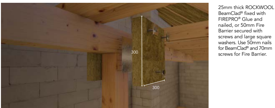
Figure 9 Nail plate protection
