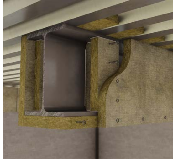
Figure 18 Tee-noggin arrangement for web depths of over 500mm. See over for Tee-noggin specification
