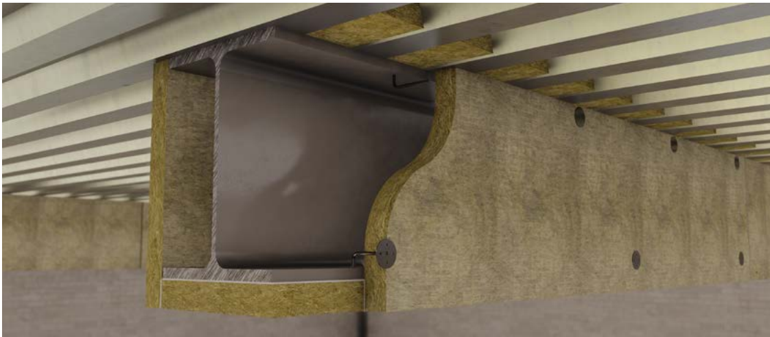
Figure 9 - Stud welded pins and board-to-board glued joints (Up to 4 hours fire protection)
