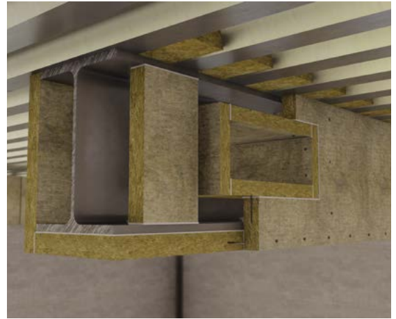
Figure 12 - Beam with square or rectangular holes (boxed and profiled protection - glued and pinned joints)
