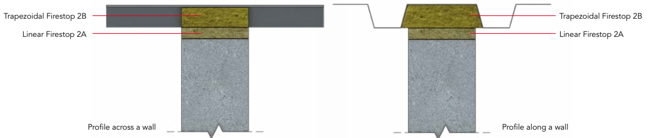
Figure 4 – Profiled metal deck over blockwork wall
