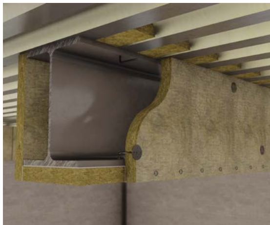
Figure 6 - Stud welded pin dry joint board system (Up to 2 hours fire protection)
