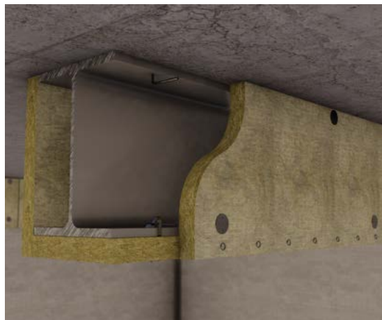
Figure 3 - Clip and stud welded pin dry joint system (Up to 2 hours fire protection)
