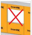
**BoardeX** joints in the window cavities should not coincide with the window edge profiles, and the joints should be fixed onto the profiles above or below the lintel.
