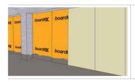
On the inside of exterior walls constructed by **BoardeX**, wet applications such as screed and ceramic coating can be carried out before screflange plasterboard. After all these wet productions are finished, **COREX** can be fixed onto the surface of **BoardeX**, and the wall surface can be finished.
