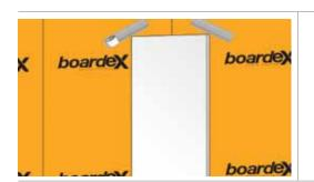
In order to reduce the risk of cracking in the corners of the door cavities, a joint tape should be applied in a cross manner and be covered by **Probase Render**.
