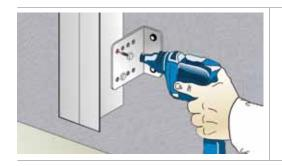
L brackets should be secured onto profiles by Drillex hex head screws from at least two points.
