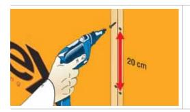
**BoardeX** should be fixed onto metal profiles by using corrosion resistant Drillex hard screws with 20 cm axle spacing.
