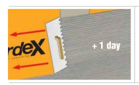
The primer coat application should be carried out at least 1 day after the joint application is completed.
