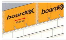
The carrier profiles of the ventilated wall systems are fixed onto the carrier profiles of the **BoardeX** exterior wall systems within the range of the axle spacings determined by manufacturing firms, and hence are designed to carry systems weighing 25 kg/m². As far as the ventilated wall systems to be applied onto **BoardeX** surfaces are concerned, the advice and application principles of the facade system manufacturers should be taken into account.
