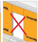
**BoardeX** joints in the door cavities should not coincide with the door edge profiles, and the joints should be fixed onto the profiles above or below the lintel.
