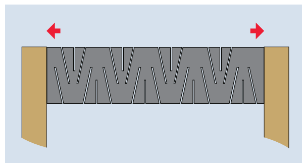
Installation of Kingspan Aerofit™ Platinum® Between Rafters
