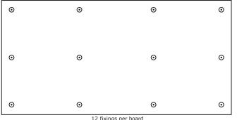
12 fixings per board (4.16 fixings / m2)
